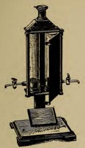
Fig. 94. WOULFF'S COLORI-METER, FOR INSPECTING ANI-LINE DYES.
