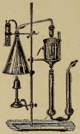
Fig. 93%. APPARATUS FOR DETERMINING THE AMMONIA IN PLANTS AND VEGETABLE EXTRACTS.
